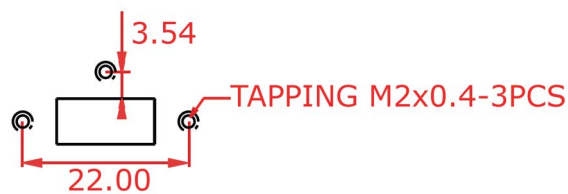
Figure 1: Threading hole dimensions for USB connectors
