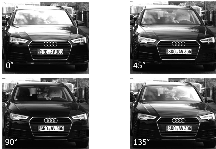
Figure 1: Polarization angle versus image brightness in sub-images
