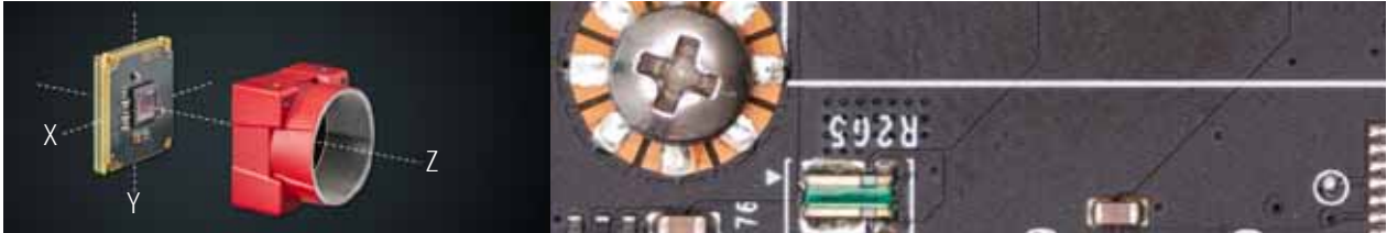
Figure 4: The sensor is accurately aligned to the optical axis of the lens
