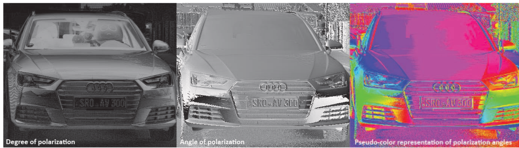
Figure 5: Degree of polarization, angle of polarization, and pseudo-color representation of polarization angles
