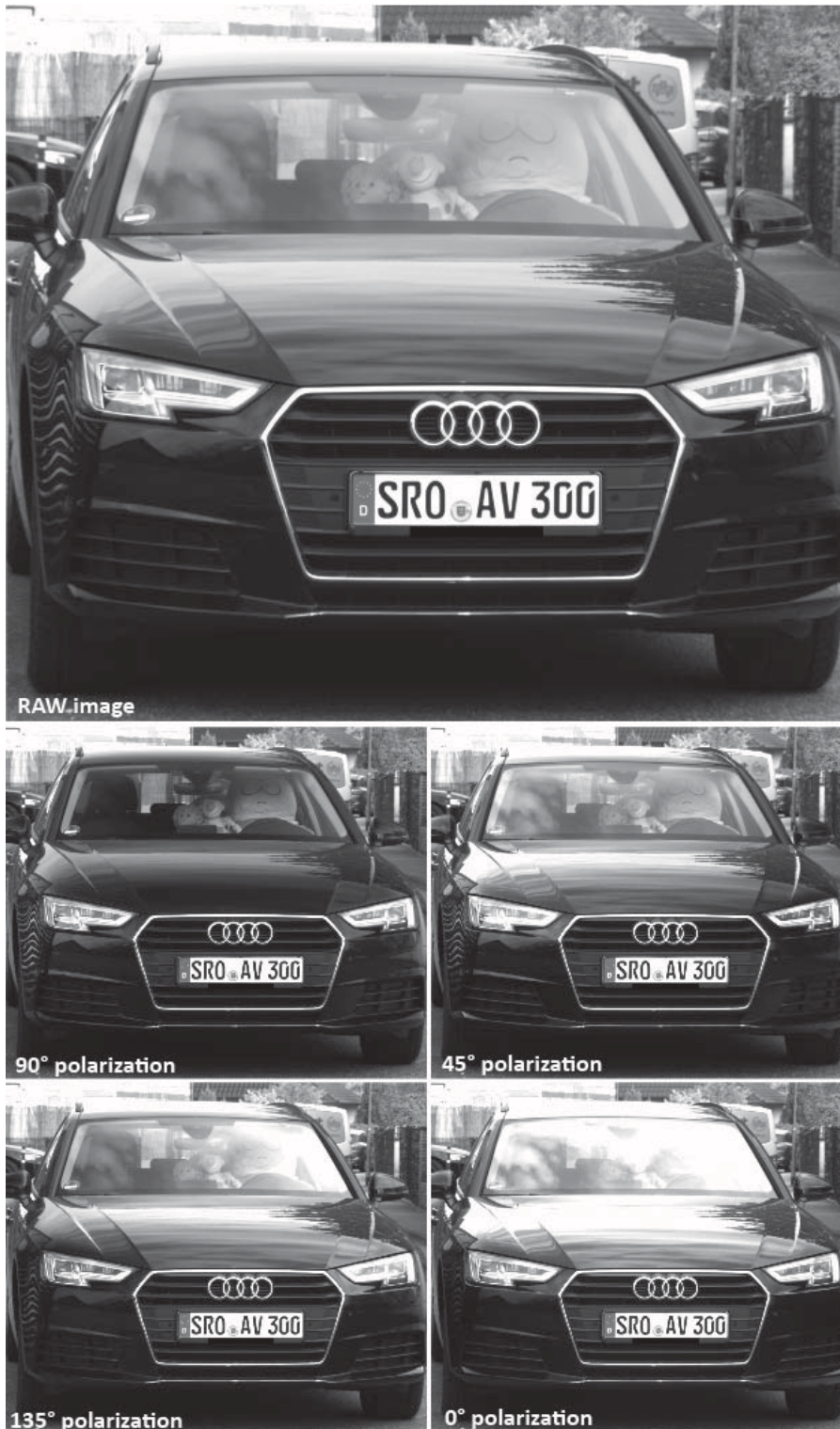
Figure 4: Sample of RAW polarization images and related sub-images of the four polarization directions
